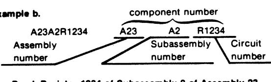
Only the circuit number will appear on the diagrams and circuit board illustrations. Each diagram and circuit board illustration is clearly marked with the assembly number. Assembly numbers are also marked on the mechanical exploded views located in the Mechanical Parts List. The component number is obtained by adding the assembly number prefix to the circuit number.
